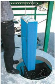
The ecoLine-b oil/water separator is designed to separate non-emulsified light liquids or low-water-soluble fluids with a specific gravity below 0.95 (gasoline, diesel, heating oils and other mineral oils) from effluent discharge. A two-step separation process, gravity separation and removal of small oil particles by coalescing media elements, produces high removal efficiencies.
