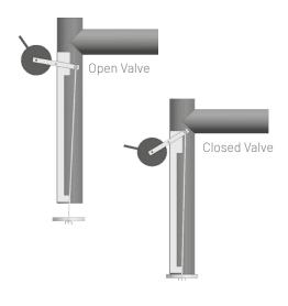
ecoLine-b separators are equipped with a spill control mechanism in the outlet pipe. The calibrated float will lose buoyancy in oil as it accumulates, hence shutting down the outlet pipe of the separator. The valve will be completely shut when the maximum oil storage capacity is reached (200mm/9inches).
